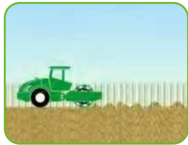
① Compact the sub base
