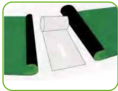
④ Roll out the seam-tape
