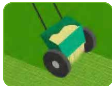
⑩ Infill silica sand (optional) and then rake or sweep
